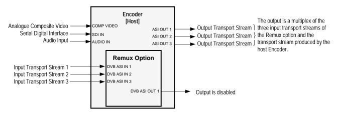
Figure 3.3: Remux Option (M2/EOM2/REMUX)
